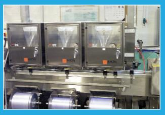
There are a trio of shrink banders (left) on each of Peak Foods' two lines; above photo shows flights that encircle the bowls to ensure positive control and a centered shrink band.
